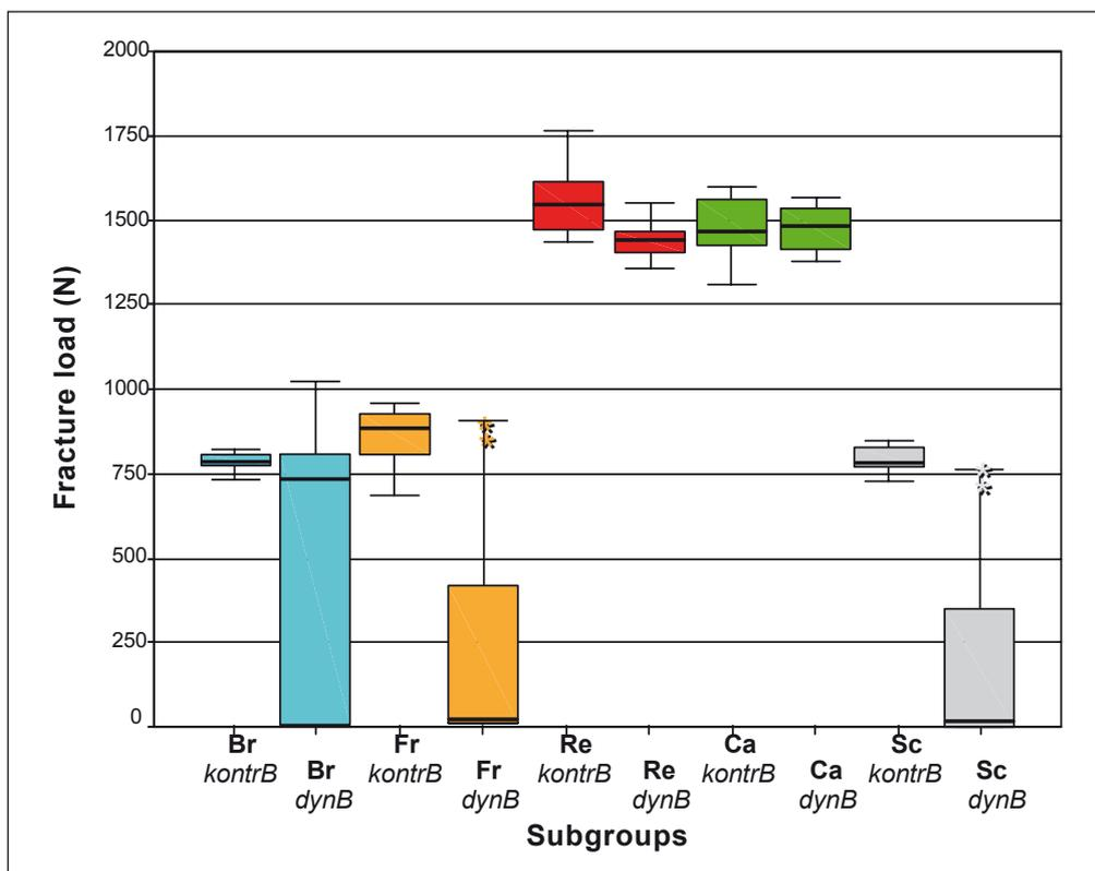
**Fig. 11** Box plot diagram of the quasi-static fracture strength values of all test groups. Br = Brånemark, Fr = FRIALIT®-2, Re = Replace® Select, Ca = CAMLOG, Sc = Screw-Vent®; kontrB = no-load control group, dynB = after chewing simulation (source: Steinebrunner 2006)
