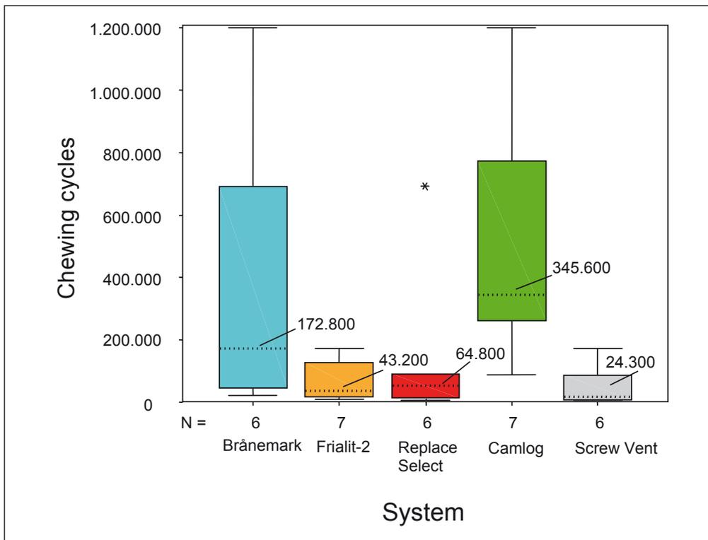
**Fig. 9** Box plot graph. The boxes show the chewing cycles reached before microbial leakage occurred in the individual systems. Each box is divided by a broken line, the median value. The value indicated by a star represents an extreme value. The CAMLOG® Implant System clearly reached the highest mean number of cycles among the tested systems (source: Steinebrunner 2006)
