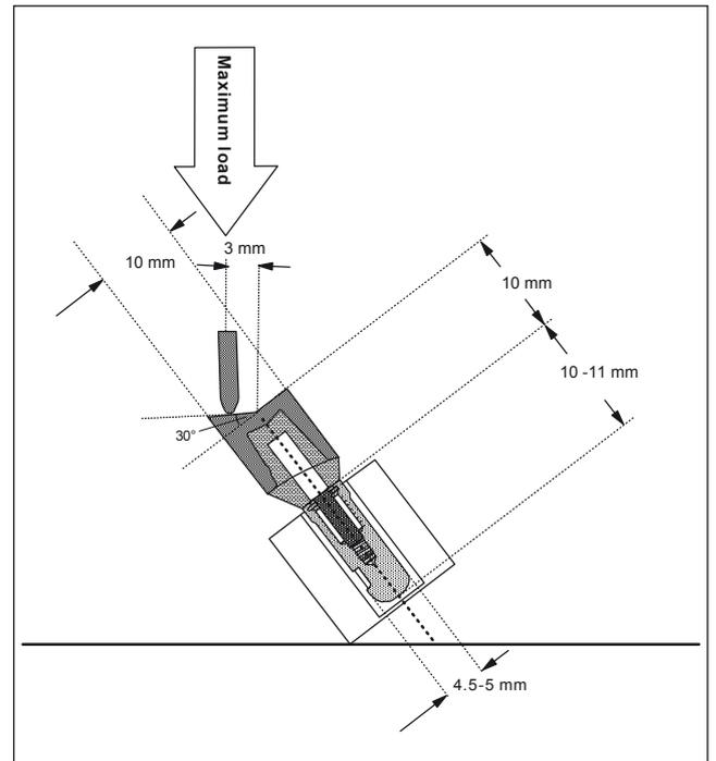
**Fig. 10** Schematic representation of the test set-up in the Zwick Z010A TN 2A universal testing machine. The force input point was identical to chewing simulation at 3 mm eccentric from the crown midpoint on the central cusp, sloped at 30° to the occlusion plane and 11.5 mm distant from the implant shoulder (source: Steinebrunner 2006)
