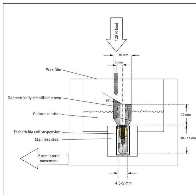
**Fig. 8** Schematic presentation of the test set-up in the multifunction chewing simulator (Willytec, Munich). This takes into account a 30° cusp slope, a 2-mm lateral movement, and the physiological vertical chewing force reported by Richter (1995) (source: Steinebrunner 2006)
