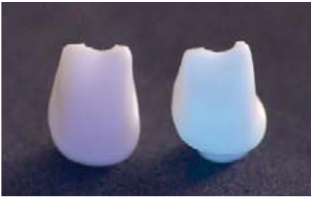
Fig. 31: The sintered abutment left (without) and right with fluorescent solution treatment.
